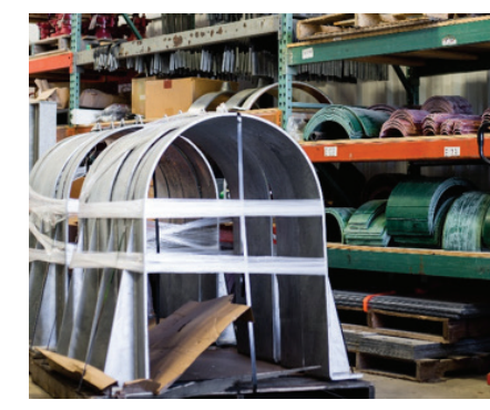
PICTURED TOP TO BOTTOM: Galvanized integrity block with pipe in, Ashland Fabrication, . warehouse
